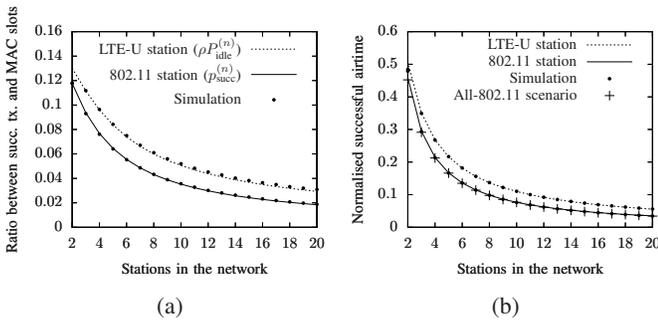
Fig. 3: Illustrating the (a) ratio between successful transmissions and MAC slots; (b) stations' successful airtime, in a network with a single LTE-U station (LBT-station) and  $\rho = \bar{\rho}$ . Network parameters are  $T = 100\sigma$ ,  $T' = T_{LBT} + \sigma$ ,  $T_{LBT} = T$ ,  $CW_{min} = 16$  and  $\bar{m} = 5$ .
