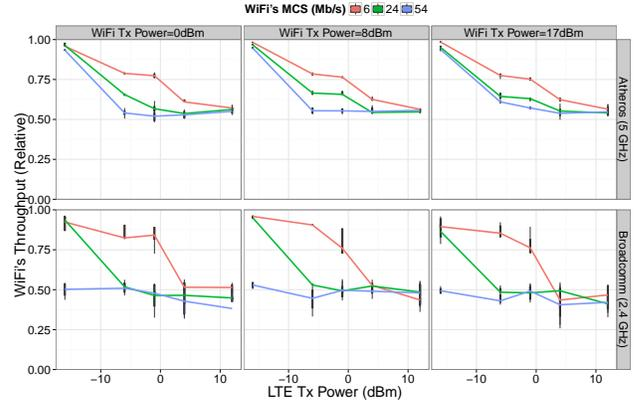
Figure 4: WiFi throughput vs. LTE transmission power
