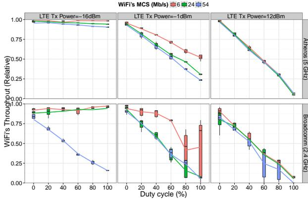
Figure 3: Impact of LTE duty cycle on performance.
