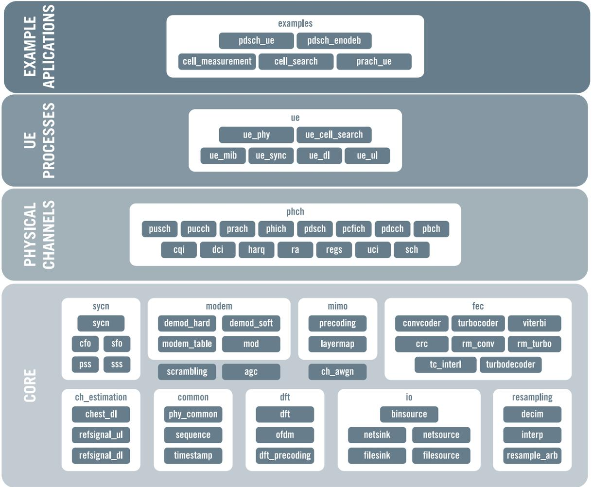
Figure 1: Module diagram for the srsLTE library.
