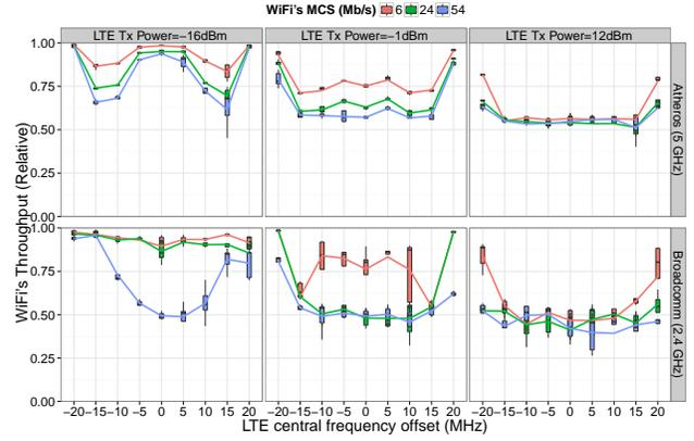
Figure 6: WiFi throughput vs. LTE central frequency
