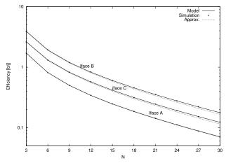
Figure 2. Overall energy efficiency of a WLAN with N stations.
